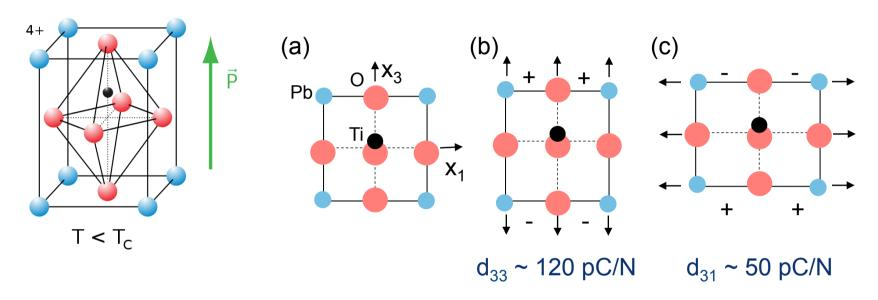
$d_{33}$ : induced polarization in direction 3 (parallel to direction in which ceramic element is polarized) per unit stress applied in direction 3 **or** induced strain in direction 3 per unit electric displacement applied in direction 3.
